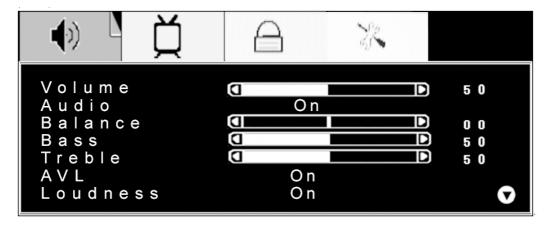
When the input source is TV mode, could select the Sound Setup, Picture Setup, Child Lock Setup, Function Setup and TV Setup. Shown in the figure below:
